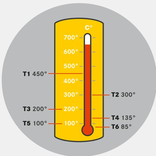
**Figure 5: European classification of maximum surface temperatures for equipment in explosion hazard zones**
