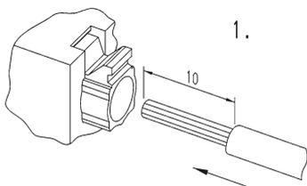
Do not twist the fine stranded wires!
